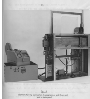
Radio 2D-paper chromatography scanner with digitization of collected data
